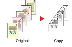
Produces two-sided copies from one-sided originals. In case of an odd number of originals, the back side of the last copy will be blank. The optional duplex unit is required.
