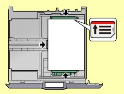
Insert the appropriate paper size card in the slot to indicate the size of the paper inside.
